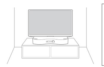
**⚠ Note:** Install on a level, stable surface. Slanted or unstable surfaces may cause the unit to fall causing damage or injury. Review safety precaution section of this manual before setup.
